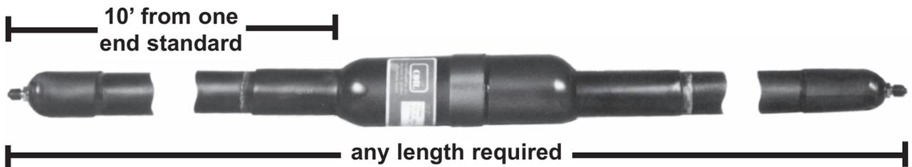
Charles Industries' C-10 type cable stubs are fully color-coded PIC cable with either ALPETH (C-10A1) or PASP (C-10B1) sheaths. C-10 cable stubs contain a gas plug 10' from one end. A STALPETH (C-10E1) version is also offered with a gas plug at 15' and standard lengths of 30' and 50'.
