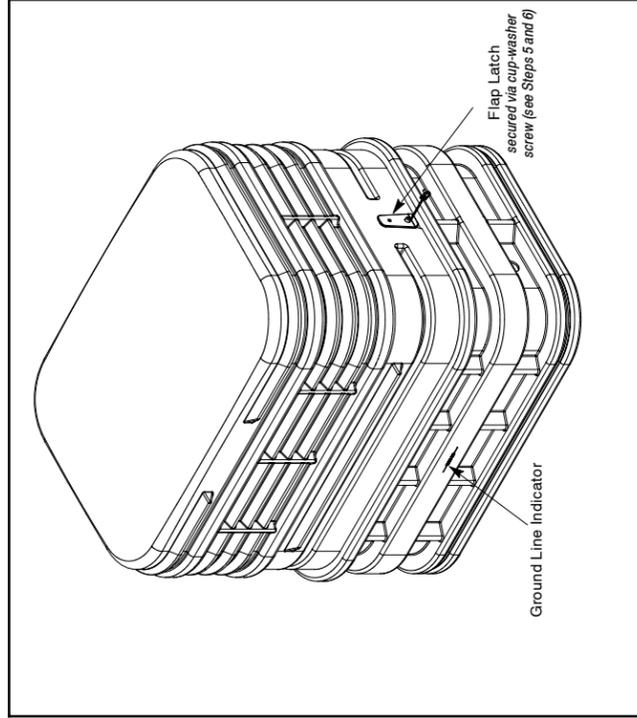
**Figure 1. Typical CMPH Enclosure, Closed View**
