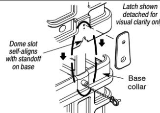
23. **Lock the CMPH.** Lock the CMPH by re-inserting and turning the cup-washer screws clockwise into the threaded holes provided for them in the standoffs. Tighten the cup-washer screws with a 216 tool or can wrench (as shown in Step 5).
