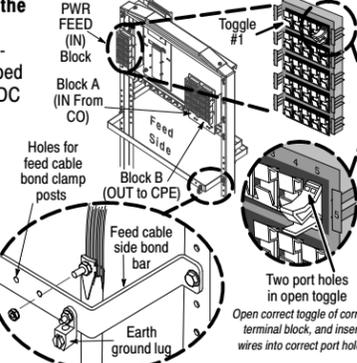
8. **Terminate power pairs.** Per company practice, terminate the first pair of the power cable at Toggle #1 in the PWR FEED (IN) block. Insert the tip wire all the way into the open toggle's left port and the ring wire all the way into the right port, then push up and back to close the toggle. Repeat and continue until all desired power pairs in the power cable are terminated.
