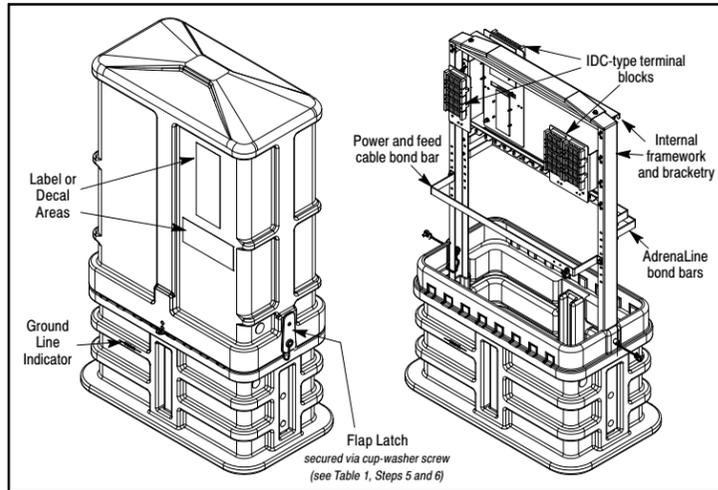
**Figure 1. Dome on and Dome off Views of CMPH-75 Enclosure, Express-Powered ADI Configuration**
