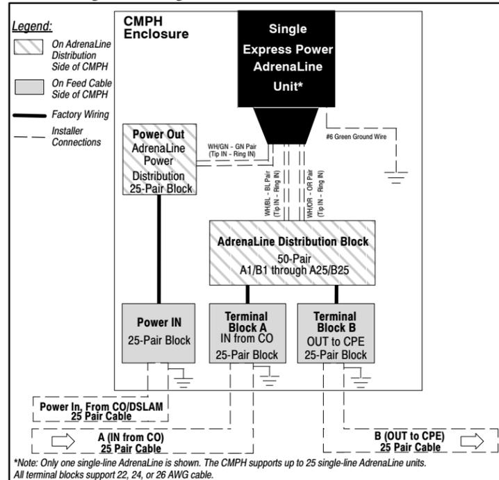
**Figure 2. Express-Powered CMPH ADI Block Diagram**
