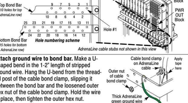
15. **Attach ground wire to bond bar.** Make a U-shaped bend in the 1-2" length of stripped ground wire. Hang the U-bend from the threaded post of the cable bond clamp, slipping it between the bond bar and the loosened outer hex nut of the cable bond clamp. Hold the wire in place, then tighten the outer hex nut.
