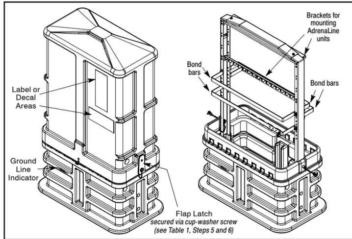
**Figure 1. Dome on and Dome off Views of CMPH Enclosure, Blockless ADI Configuration**
